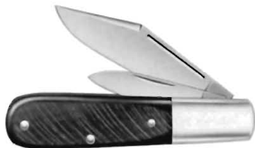
NO. 822 BARLOW KNIFE — Carbon steel blades and springs. Solid nickel-silver bolsters and brass scales. Saw pattern Delrin handle. Master clip blade and pen blade. Knife has traditional jack-knife blade action with square tangs on both blades to stop them in the half-open position. Length closed 3 3/4".
