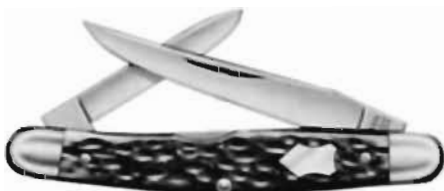
NO. 652 LARGE PEN KNIFE — Carbon steel blades and springs. Stag pattern Delrin handle. Knife is designed with blade at each end operated by a single spring to make it slim and light weight. Long clip master blade and pen blade. Length closed 3 3/8".
