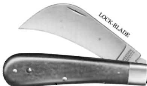
NO. 854 UTILITY KNIFE — Carbon steel blade and spring. Brown Delrin handle has hole for chain or thong. Flat ground 2 3/4" blade. Split-scale type lock holds blade open when in use. Blade has square tang. Length closed 4".
