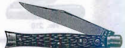
No. 150 Safety Push Button Knife, Light Hunting Knife Pattern, 4 inches long; Staggered Handles; Slim Clip Blade; Brass Linings; Nickel Silver Bolsters and Caps; Blade Polished on one side. Weight Per Dozen, 1 lb., 8 oz.
