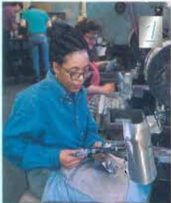
INDIVIDUAL INSPECTION, PART OF EVERY OPERATOR'S JOB. (Joanna and Cindy) Detect defective material or faulty operations. A variety of gauges and hand tools are supplied to insure that all inspection standards are met.
