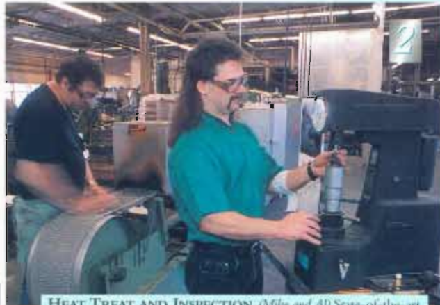
HEAT TREAT AND INSPECTION (Mike and Al) State-of-the-art heat treating equipment is used to insure blades are the absolute hardness for holding an edge but not compromising ability to re-sharpen. Rockwell, Tinsley and grain size checks are made on every job. History is kept to maintain accurate records.
