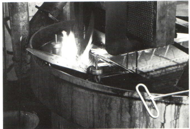
Steel used for blades are hardened by immersing in hot lead bath and quenched in oil solution.
