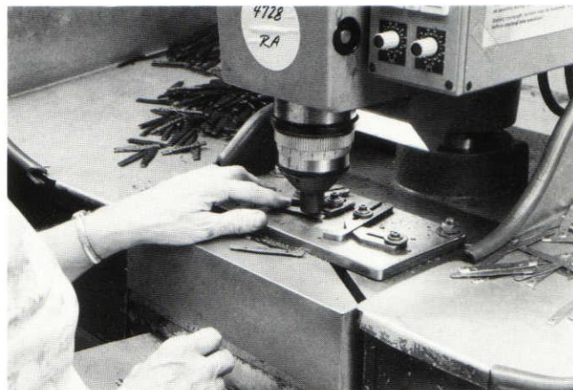
Covers and liners are united . . . ready for riveting.
