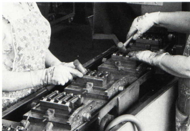
Loading assembled knives into machine for grinding and polishing of spring backs.
