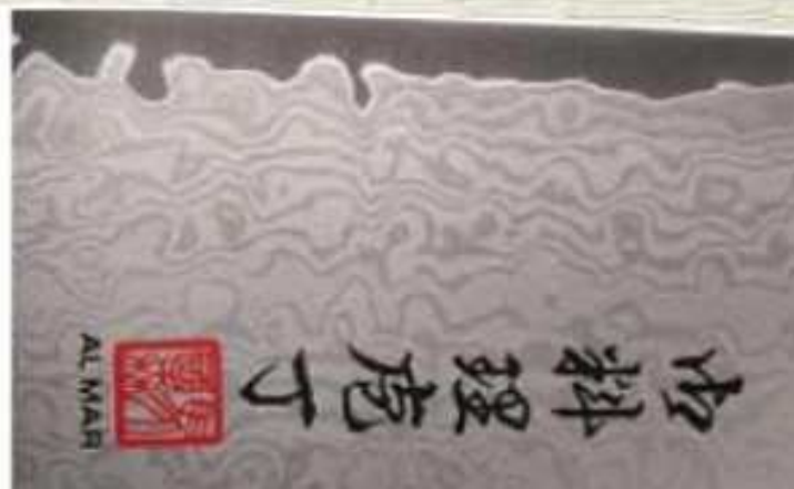
Ultra-Chef blade showing - the detailed pattern in the multiple layers of steel.
